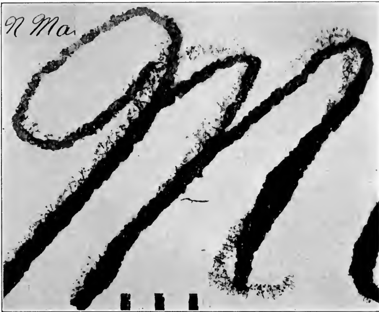
FIG. 32—Illustration made to show pencil outline of letter covered and partly covered with ink. Actual size and enlarged x 13.
